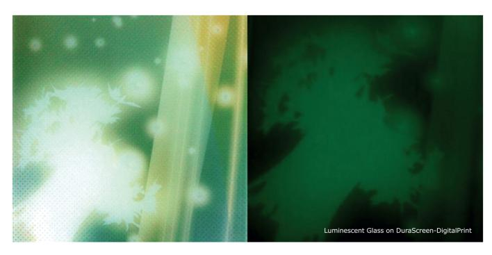
SSG® Luminescent Glass illuminates in the dark. It is the result of glass combined with luminous coatings to give a special visual effect in the absence of light. The special coating gets energised by normal lighting to glow in the dark. SSG® Luminescent Glass is available in heat-strengthened, tempered on clear or tinted glass substrates either in full coat or custom patterns. Coloured versions can also be achieved with colour PVBs in laminated glass.
